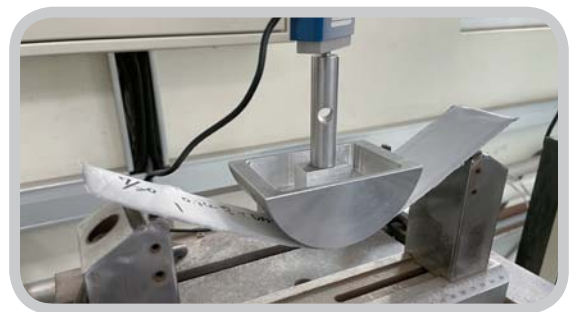
Tile adhesive transverse deformation test (EN-12002) 磁磚接著砂漿柔軟性測試 (EN-12002)
