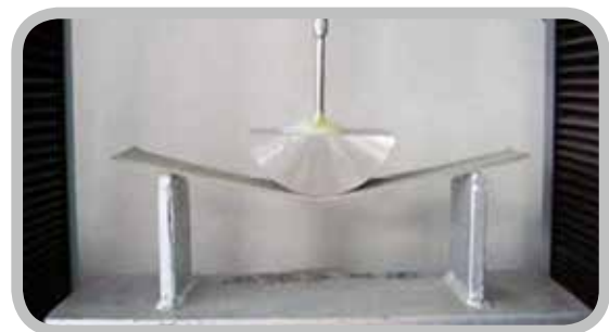
Tile adhesive transverse deformation test (EN-12002) 磁磚接著柔軟性測試 (EN-12002)
