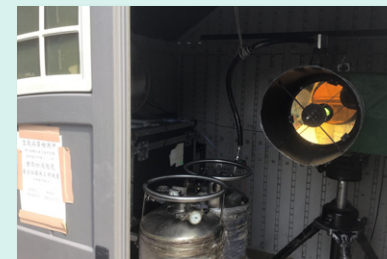
▲ Open-Path Fourier Transform Infrared Emitter
