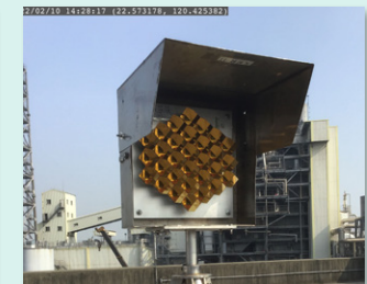
▲ Open-Path Fourier Transform Infrared Receiver
